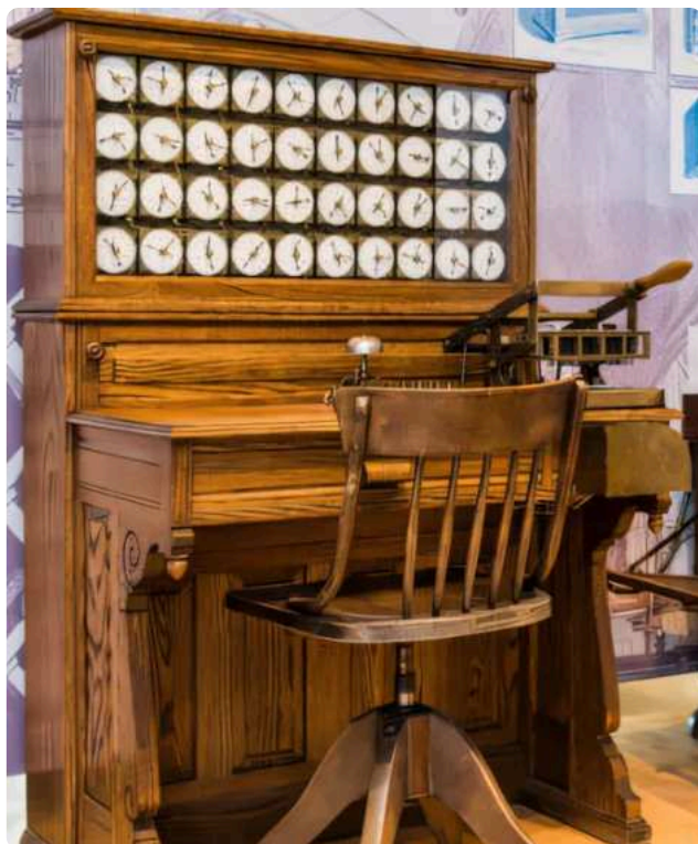
Hollerith's tabulating machine (1890), the first device capable of automatically calculating means from large datasets
